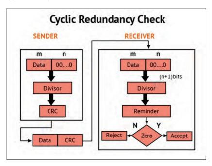
Fig. 7.4.4 Cyclic Redundancy Check
