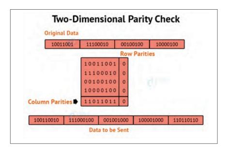
Fig. 7.4.2 Two-Dimensional Parity Check
