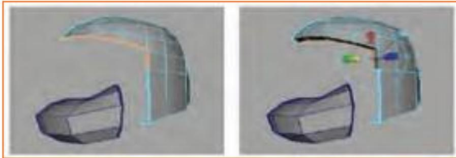
Fig.6.4.35: Extrude the Top and Side Edges Inwards
