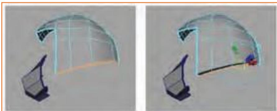
Fig.6.4.34: Extrude the Top and Side Edges Inwards
