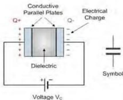
The plates store the energy of the electrons as electrical charge on, which means, greater the plates and lesser the distance, more will be the capacitance.
