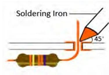
Step 7: Touch the solder to the iron tip and move that around the joint by keeping the iron tip fixed. Let the solder melt and flow till the joint is covered, as shown in the following figure:
