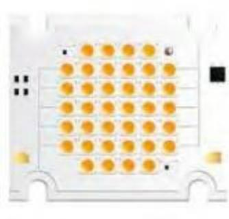
LED based light engine module
