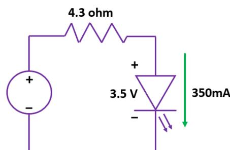
Indicator LEDs are generally powered by this method. For lighting applications, there are some drawbacks of this method and one of them is inefficiency. There is loss of power across the resistor in the form of heat. For example, if a 10V source is used to provide power
