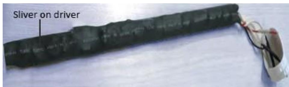
7. Place the sleeved driver inside the aluminium extrusion, and solder the input wires to the end caps and the output wires to the light engine input points.
