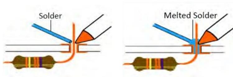
Step 8: Remove the iron after removing the solder and make sure the joint is kept stationary till it cools down.
