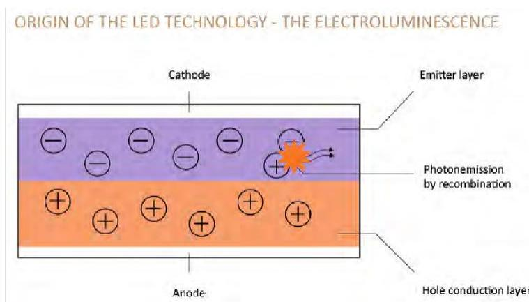
In LED chips, on application of certain voltage, electromagnetic radiation in the form of light is given out.
