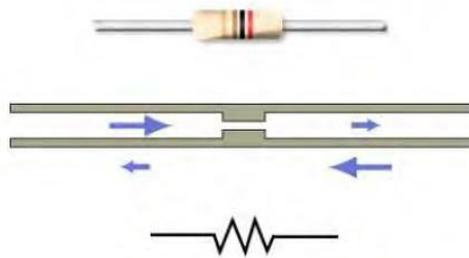
Resistance is measured in Ohms ( $\Omega$ )  $1000\Omega = 1\text{k}\Omega$ ,  $1,000,000\Omega = 1\text{M}\Omega$
