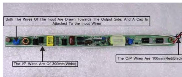
6. Take the tested driver and insert into the sleeve. Pass the sleeved driver through the reflow oven at conveyor speed 0.70 m/min, for heat shrinking of heat sink sleeve at reflow temperature of 110 degree C.
